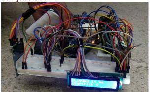
Figure 4: Proposed System with LCD, RFID, Arduino Mega
