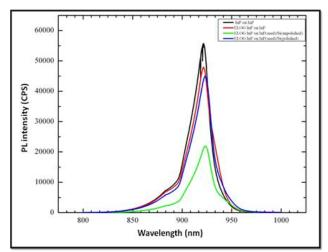
Figure 2: Room temperature Photoluminescence spectrums of ELOG InP and InP/InP planar substrates
