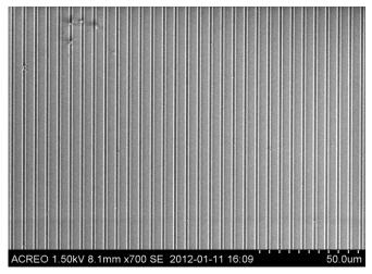
Figure 1: Surface morphology of SEM pattern on the Fe-InP substrate
