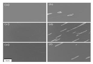
Figure 4: (a) and (b) SEM micrographs of ELOG InP on InP patterned substrate,
