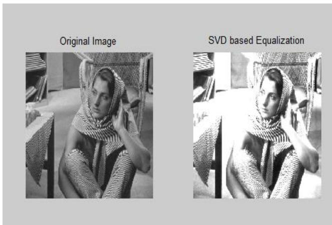
Fig 4.5 Results of Singular Value Equalization (a) Original Image (b) Image obtain using SVE Technique
