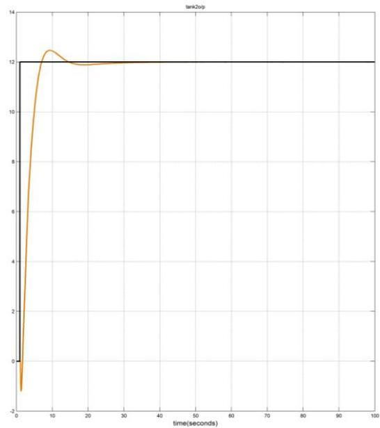
Figure 9: 1-2/2-1 Control Paring O/p response of Tank2
