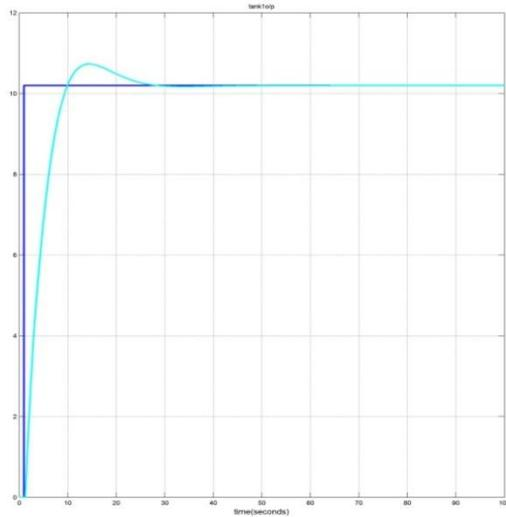
Figure 5: 1-1/2-2 Control Paring O/p response of Tank1
