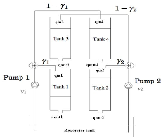
Figure1: Schematic Diagram of Quadruple Tank Process
