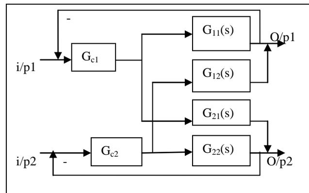
Figure 4: 1-1/2-2 Control Paring Block Diagram
