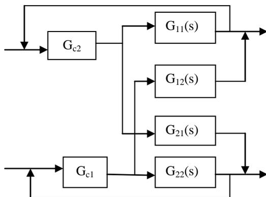
Figure 7: 1-2/2-1 Control Paring Block Diagram
