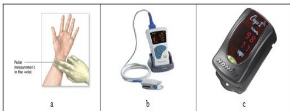
Figure: 2 (a) A manual pulse measurement [27], (b) portable hand-held pulse oximeter [28] and (c) Nonin's Onyx II finger clip Bluetooth oximeter [29].
