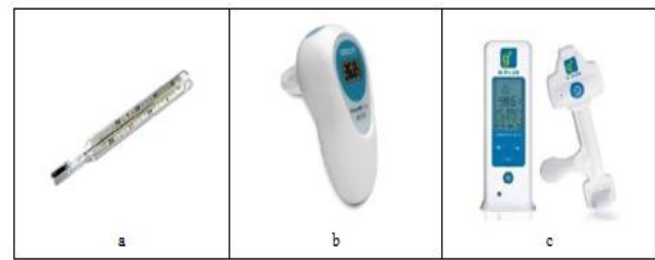
Figure:3 (a) A mercury in glass thermometer [31], (b) The Omron's instant ear thermometer measurement device [32] and (c) The G-plus wireless remote body temperature used for continuous body temperature measurement [33].
