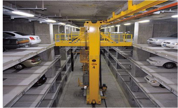
Figure 1: Integrated Car Parking Solutions
