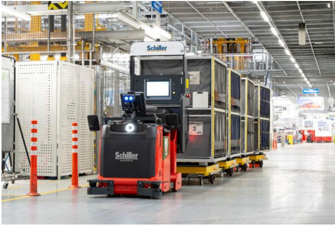
Figure 6: Autonomous vehicles delivering parts around the factory [11].
