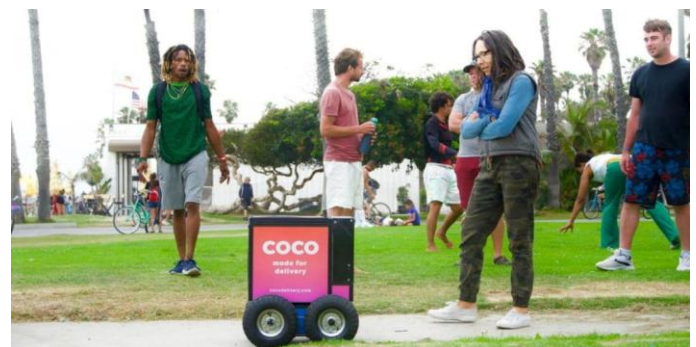
Figure 8: Coco remote-controlled delivery robot [12].
