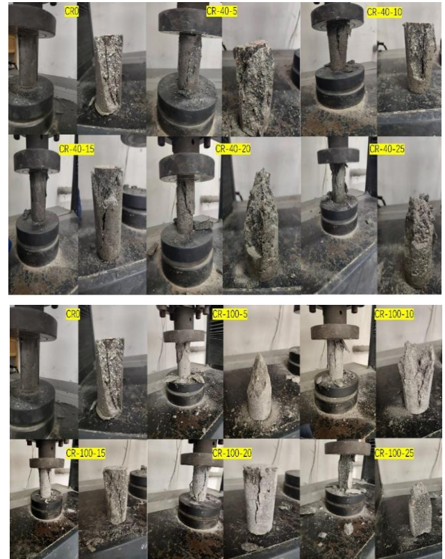
Fig. 6 Damage patterns of rubber mortars with different particle sizes and dosages under compression
