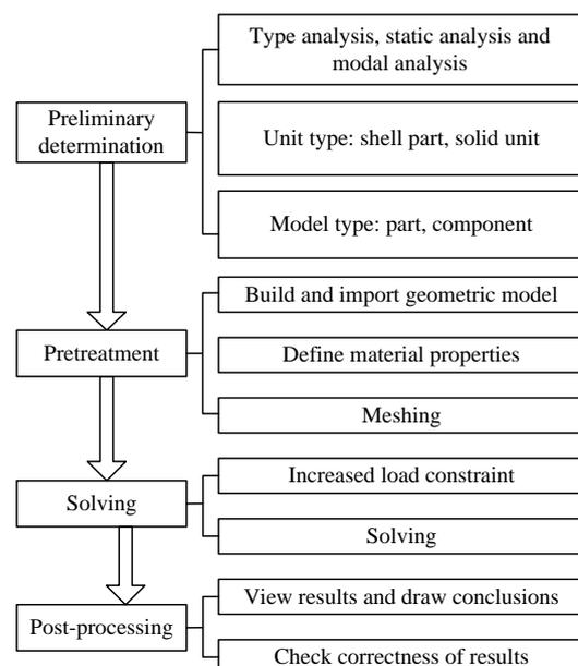
Figure. 2 Basic flow chart of static analysis
