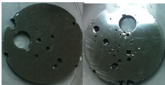
Fig. 9 Pits generated on the surface of (a) Stellite 6B, (b) Stellite 6K after 6 day immersion in Green Death solution at 60°C.
