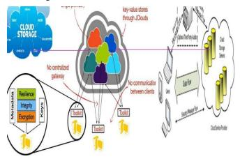
Figure 3. Architecture Design of the Secured Public Data in the Database of Cassandra
