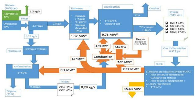
Fig.3 Diagram of the new hybridsolid waste treatment, from sorting to electricity generation
