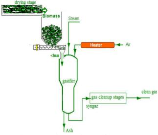
Fig.1Schema of trained flow gasifier [6]
