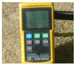
Fig.4. K-Type data logger.
