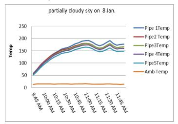
Figure 8. Air temperature inside tubes with reflectors.
