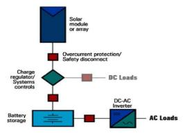
Figure 2: Standalone Photovoltaic System
