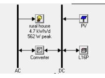
Figure 3: Homer Schematic Diagrams for the PV System
