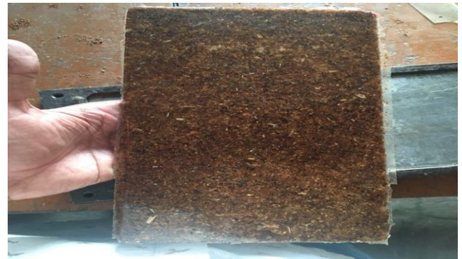
Figure 5: Composite Made With Rise Husk
