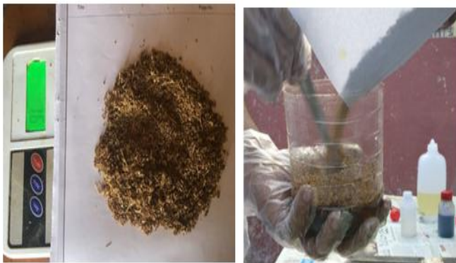
Figure 3: Measuring And Mixing Of Rice Husk With Resin
