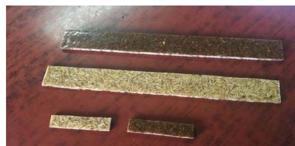
Figure 6: Specimen Used For Tensile Test and Impact Tests
