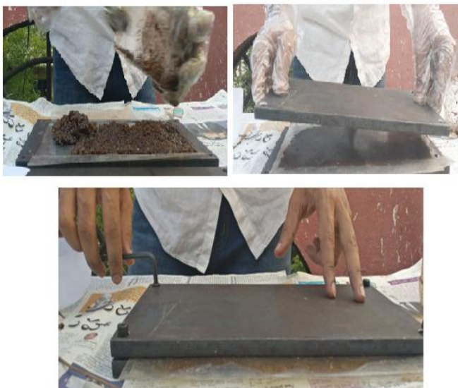
Figure 4: Filling and Closing The Die
