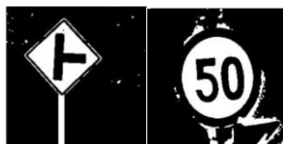
Fig. 6. Segmentation of warning signs
