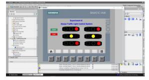
Figure 12: When timer3 is time up, the Red1, Yellow2, Red3 and timer4 are on
