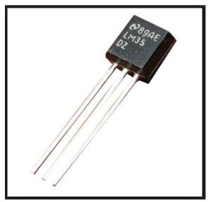
The LM35 series are precision integrated-circuit temperature devices with an output voltage linearly proportional to the Centigrade temperature. The LM35 device has an advantage over linear temperature sensors calibrated in Kelvin, as the user is not required to subtract a large constant voltage from
