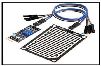
The rain sensor module is an easy tool for rain detection. It can be used as a switch when raindrop falls through the raining board and also for measuring rainfall intensity. The module features, a rain board and the control board that is separate for more convenience, power indicator LED and an adjustable sensitivity though a potentiometer.
