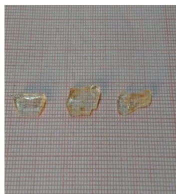
Figure : 1 Grown crystal of LS
