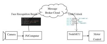
Figure 1: Block Diagram of Face Recognition Door Lock System
