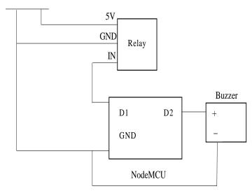
Figure 3: Circuit Diagram of Lock/Unlock System with NodeMCU
