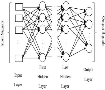
Figure 8: Architecture of a Back Propagation Neural Network
