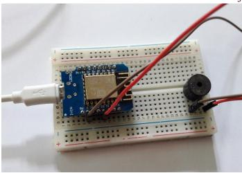
Figure 4: Hardware of Lock/Unlock System with NodeMCU
