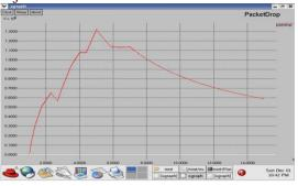
In the above Fig shows that Packet Loss. Packet Loss is where network traffic fails to reach its destination in a timely manner. Most commonly packets get dropped before the destination can be reached.
