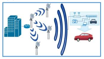
Fig. 6. A Point to Multipoint Access Point Connectivity
