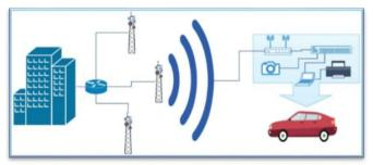
Fig. 5. An Extended Service Set Access Point solution
