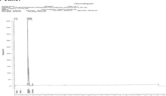
Figure 4 GC analysis for the oil extracted by steam distillation method for sample sugarcane.
