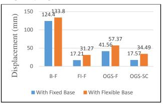
Fig.3.2: Top storey Displacement for different Structural forms
