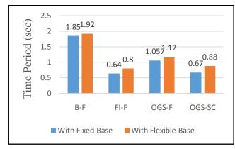
Fig.3.4: Modal Time Period for different structural forms
