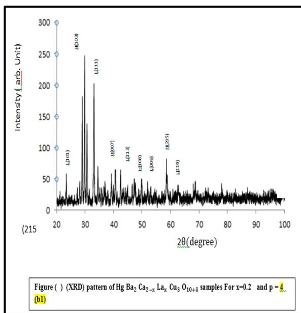
Figure ( 5 ) (XRD) pattern of  $\text{Hg Ba}_2\text{Ca}_{2-x}\text{La}_x\text{Cu}_3\text{O}_{10+\delta}$  samples For  $x=0.2$  and  $p = 6 \text{ ton/cm}^2$
