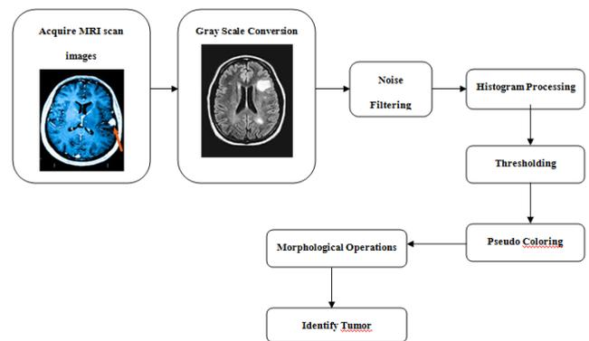
Fig. 3 The proposed – Thresholding based Brain Tumor Detection System
