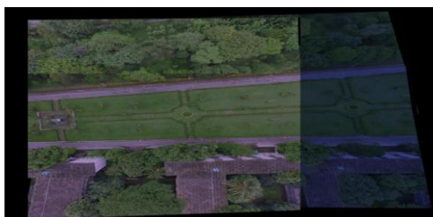
Fig. 15. Mosaic image with SIFT + RANSAC algorithm for Fig. 7, Fig. 9, Fig. 11 and Fig. 13
