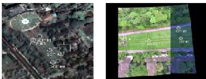
Fig. 18. Condition 2, GCPs with indistinct location on reference image and distorted image with non-parametric approach
