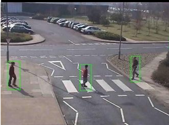
Fig.10 Extraction of a frame after removal of shadow by morphological dilation
