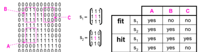
Fig. 2 Fitting and hitting of a binary image with structuring elements s_1 and s_2 .
