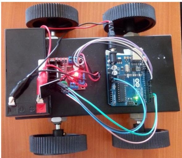
Figure 4: Proposed System with, Arduino Uno, ESP8266
