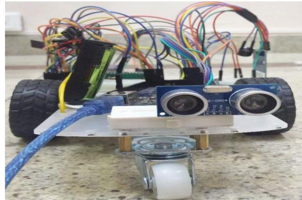
Figure 5: Proposed System with Ultrasonic Sensor
