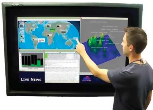
Figure 5: The Assessment Wall consists of linked interactive visualizations for streaming text documents on a high resolution touch-screen interface.
