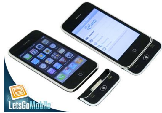
Figure 6: RFID Chip reader attached to mobile phones
