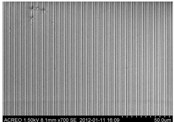
Figure 1: Surface morphology of SEM pattern on the Fe-InP substrate
