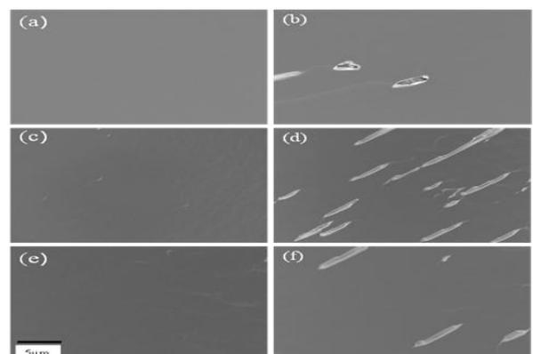
Figure 4: (a) and (b) SEM micrographs of ELOG InP on InP patterned substrate,
