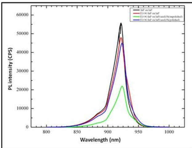
Figure 2: Room temperature Photoluminescence spectra of ELOG InP and InP/InP planar substrates
