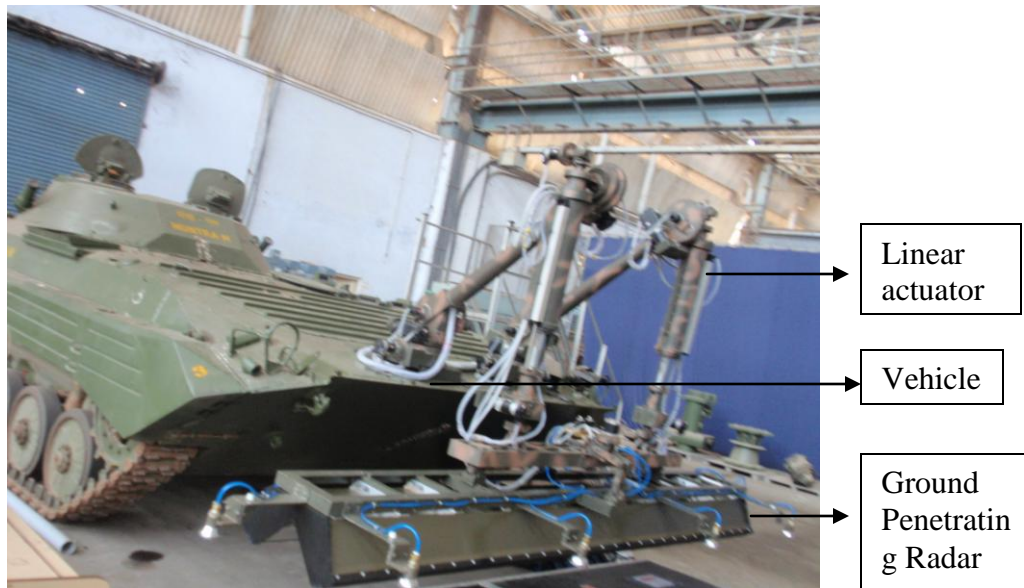
Figure 13 Integrated view of GPR in Robotic arm
