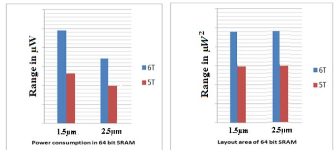
Figure 10: Comparisons between 64 Bit 6T and 5T SRAM
