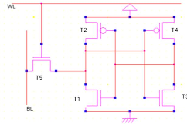
Figure 2: 5T 1Bit SRAM (proposed)
