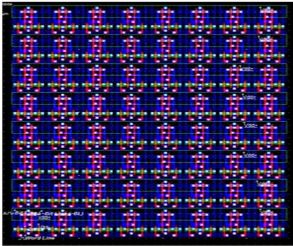
Figure 8: Layout Design of 64-BIT 6T SRAM by Using 2.5µm Technology by Microwind software
