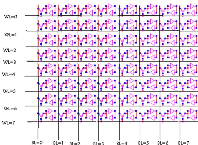
Figure 5: Block diagram of 5T 64-bit SRAM
