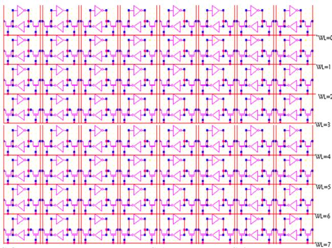
Figure 4: 64-BIT 6 T SRAM
