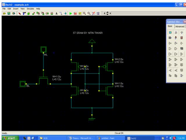
Figure 3: Schematic of 5T 1-Bit SRAM by DSCH2
