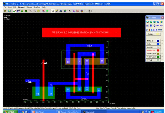
Figure 7: Layout Design of 1-Bit 5T SRAM by Using 1.5µm Technology
