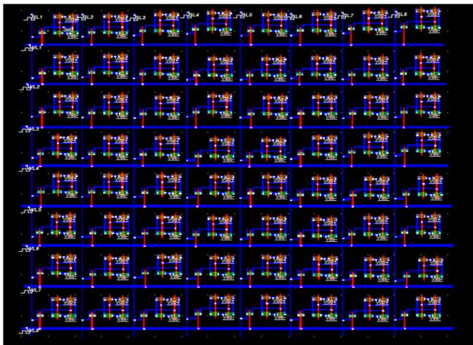
Figure 9: Layout Design of 64-BIT 5T SRAM by Using 2.5µm Technology by Microwind software
