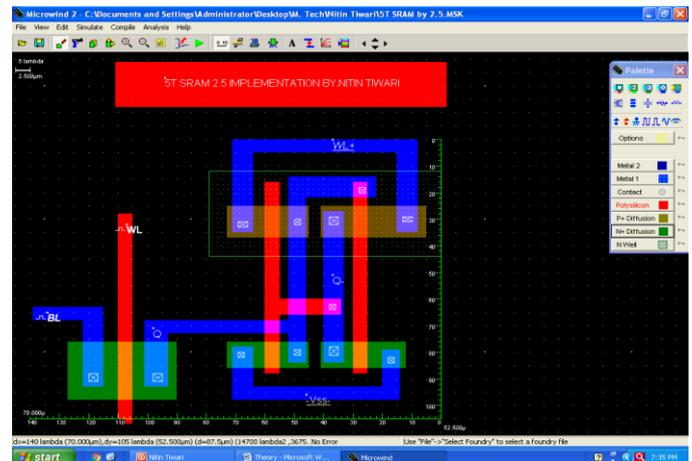
Figure 6: Layout Design of 1-Bit 5T SRAM by Using 2.5µm Technology
