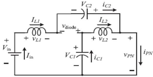
Figure 3: Equivalent Circuit of QZSI in Shoot through State
