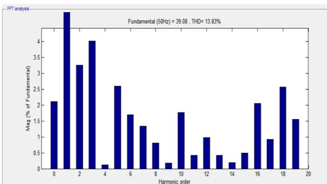
Figure 10: THD for seven-level inverter with MPC
