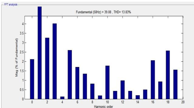
Figure 10: THD for seven-level inverter with MPC
