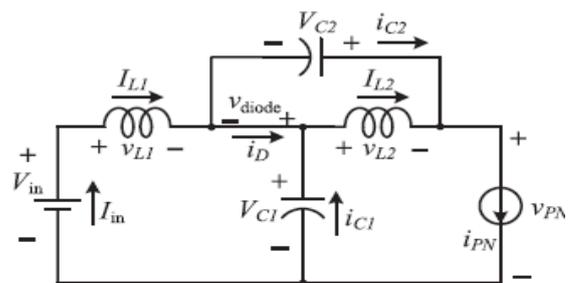
Figure 2: Equivalent circuit of QZSI in Non-shoot through state
