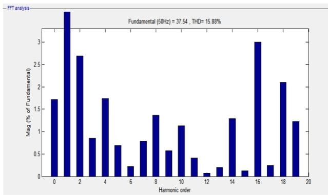
Figure 9: THD for seven-level inverter without MPC
