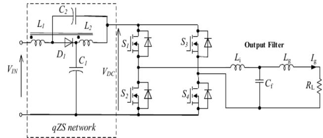
Figure 1: Equivalent circuit of single- phase QZSI
