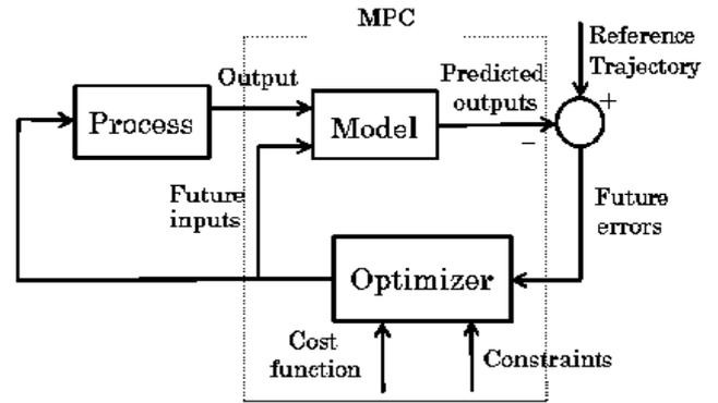
Figure 4: Block diagram of MPC
