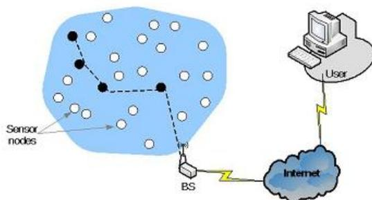
Figure 1: Architecture of a Wireless Sensor Network
