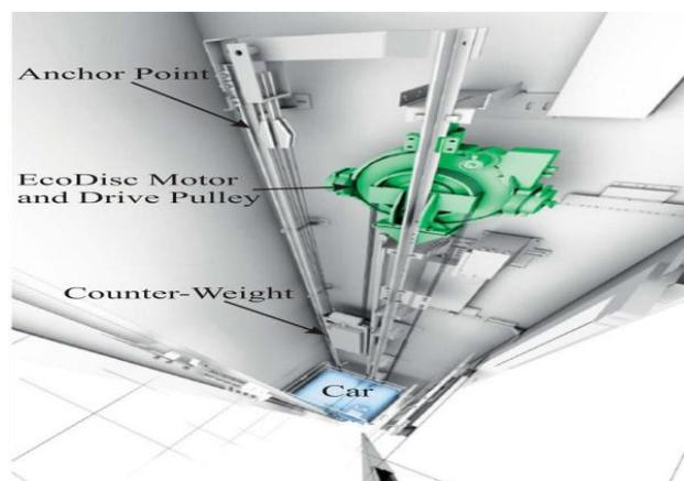
Figure 2: Kone Machine-Room-Less Elevator System [3]
