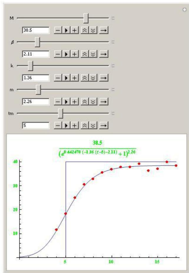
Figure 9: The appropriate fitting of experimental data by the shifted Stannard growth function  $S_m^*(t)$  with  $M = 38.5$ ,  $\beta = 2.11$ ,  $k = 1.36$ ,  $m = 2.26$ ,  $t_m = 5$ .
