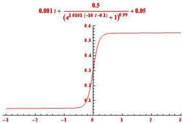
Figure 7: 6-parameters Stannard growth function (6) with:  $k = 10$ ,  $m = 0.99$ ,  $\beta = 0.1$ ,  $a_1 = 0.05$ ,  $b_1 = 0.001$ ,  $a_2 = 0.5$ .
