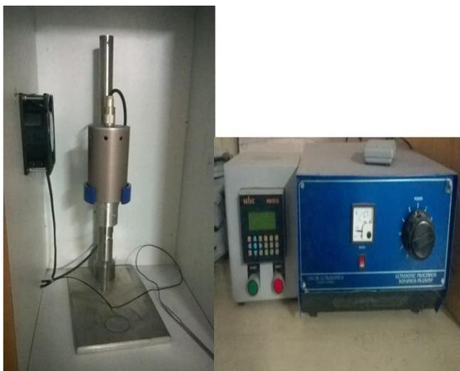
Figure 3: Photograph of Ultrasonic Probe Machine Used for nanofluid Preparation
