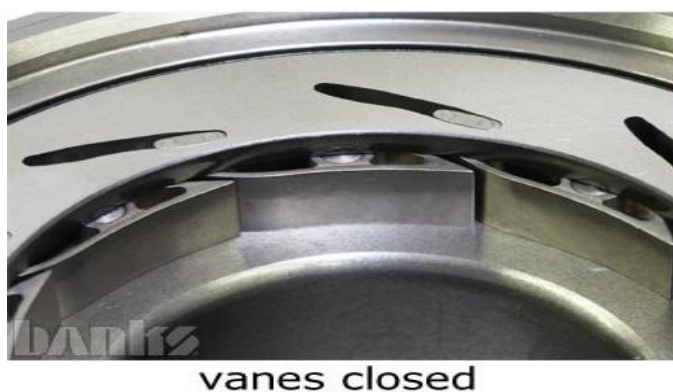
Fig. 9 Open and Close angle of vanes
