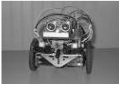
Fig.8 Front view of the robotic vehicle and ultrasonic sensors
