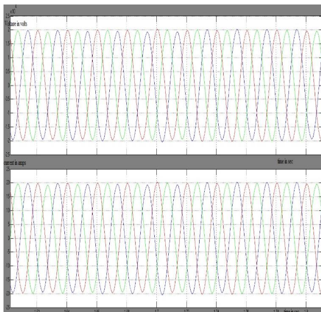
Fig 8: Output Voltage and Current of Inverter
