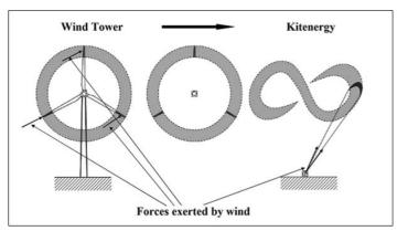
The kites are flown on a predetermined trajectory, that can transform the exerted force on the cable, to an overall mechanical torque which rotates the vertical axis turbine. About twenty automatically controlled kites can keep rotating a turbine of 1,600 meters diameter at a speed of 15 revolutions per hour. This can generate 1 Gigawatt of power, equivalent to a medium size nuclear power station
