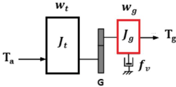
Fig.2. mechanical system of a DFIG wind turbine.
