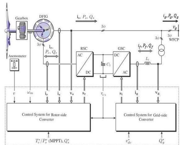
Fig.1. Block diagram of the digital control scheme for BTB VSC-based DFIG WECS.
