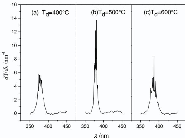
Fig.3 Curves of variation of  $dT/d\lambda$  with wavelength of ZnO thin films grown at substrate temperatures of 400, 500 and 600°C
