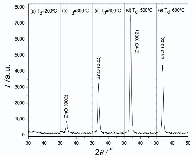
Fig.1 XRD spectra obtained from ZnO films deposited at substrate temperatures of (a) 200, (b) 300, (c) 400, (d) 500, (e) 600 °C
