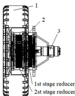
Fig.1 Working Principle Diagram of Wheel Side Reducer
