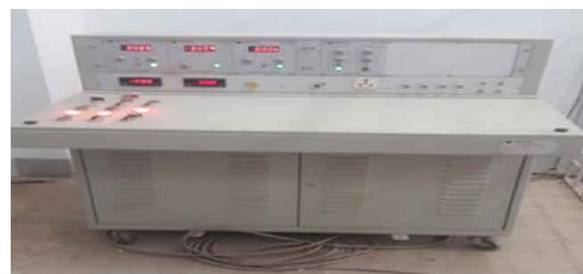
Fig. 5. Control desk of high voltage laboratory
