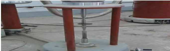
Fig. 6. Sample between the two electrodes during dielectric strength test
