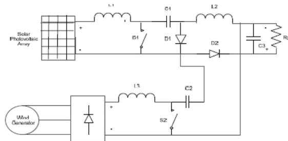
Fig. 6. DC-DC Converter - 5
