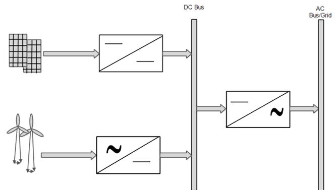
Fig.1. General Power Conversion method for combined Solar energy systems connected to DC and AC grid
